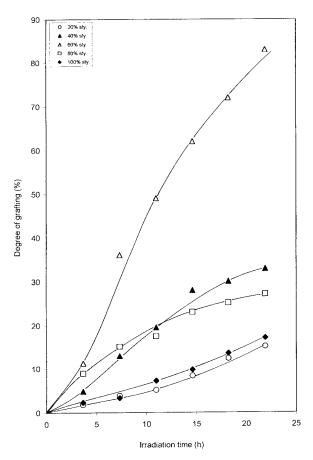
**Figure 1** The degree of grafting–time curves at various styrene concentrations (20-100 vol %), in dichloromethane as a diluent, in nitrogen atmosphere, at room temperature, and at a total irradiation dose of 20 kGy.
