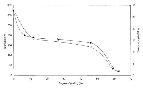
**Figure 8** Tensile strength  $(\bigcirc)$  and elongation percent at break  $(\bullet)$  vs. degree of grafting (%) of PFA-g-polystyrene films.
