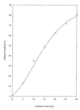
**Figure 3** The degree of grafting (%) of styrene onto PFA vs. irradiation dose (kGy) at a dose rate of 0.37 G/s.
