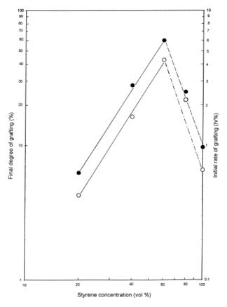
**Figure 2** Logarithmic plot of the initial rate of grafting  $(\bigcirc)$  and the final degree of grafting  $(\bullet)$  vs. styrene concentration (vol %); the same conditions as in Figure 1.
